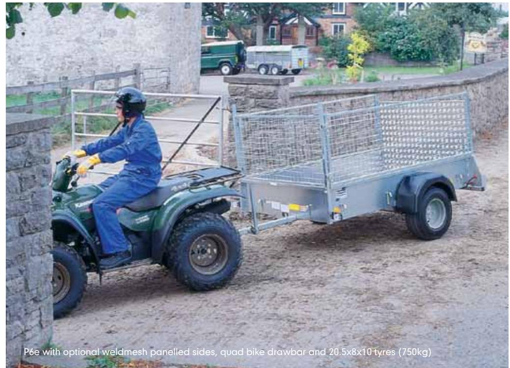
P6e with optional weldmesh panelled sides, quad bike drawbar and 20.5x8x10 tyres (750kg)
