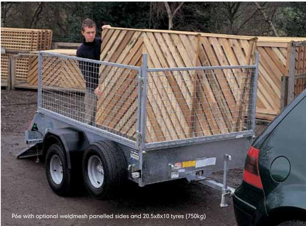
P6e with optional weldmesh panelled sides and 20.5x8x10 tyres (750kg)
