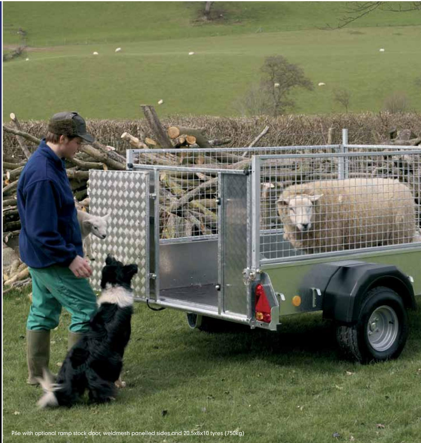
P6e with optional ramp stock door, weldmesh panelled sides and 20.5x8x10 tyres (750kg)
