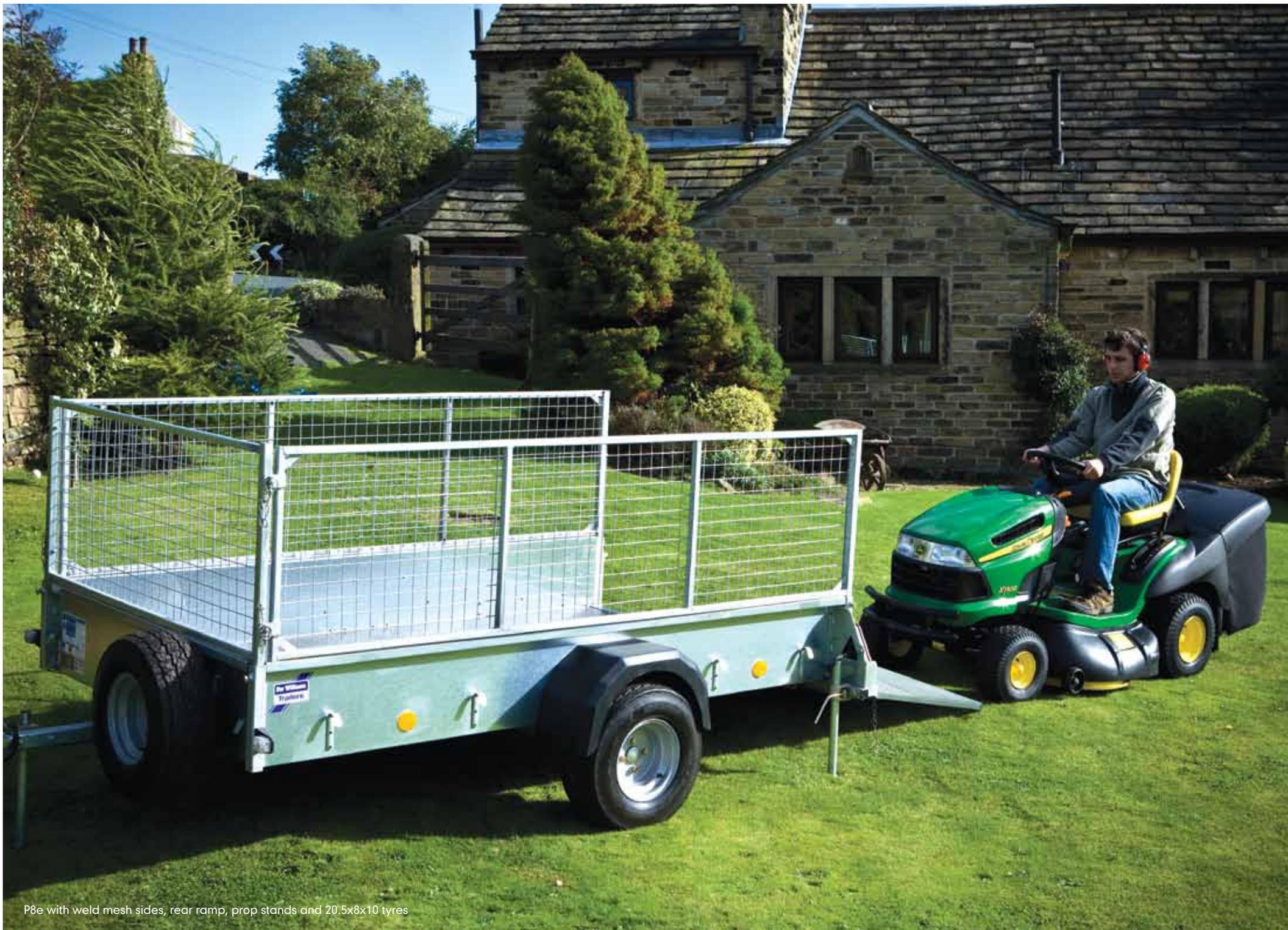
P8e with weld mesh sides, rear ramp, prop stands and 20.5x8x10 tyres
