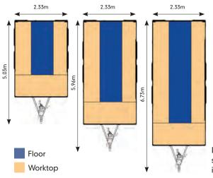
Drop floor and worktops showing dimensions of internal features.
